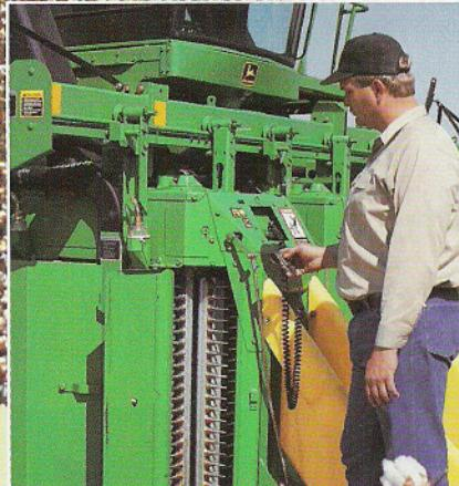
**Inspect or lube from ground level.** A tethered control lets you rotate and lube the picking units from the ground. The proven onboard lubrication system completely lubricates picking units.
