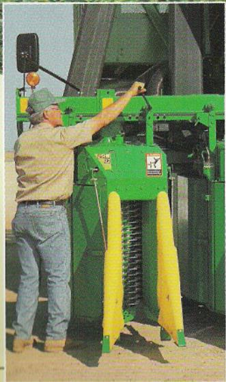
Adjusting the unit spacing on a new John Deere 9976 is a fast, easy, one-person job. Simply pull a pin and crank the unit into place. And with the narrow profile of the PRO-SERIES row units, you've got plenty of elbow room for accessing the doffers and moistener pads for cleanout.
