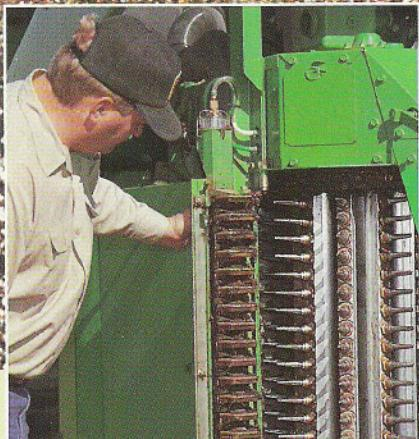
**All-new row-unit service convenience.** Both the PRO-12 and PRO-16 row units feature swing-out moistener columns for quick inspection, fast adjustment, and easy moistener pad replacement.
