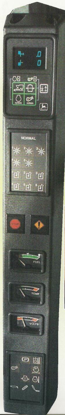
*A dual digital readout provides engine and fan speed, moistener-system pressure, and oil temperature. Any problem with the picking units, such as plugging, are identified quickly with Harvest System monitors. Additional monitors alert you to problems with hydraulic/hydrostatic oil temperature, air filter restriction, engine oil pressure, and engine coolant temperature. There's even an indicator that tells you when all the conditions have been met for operating the remote tether.*
