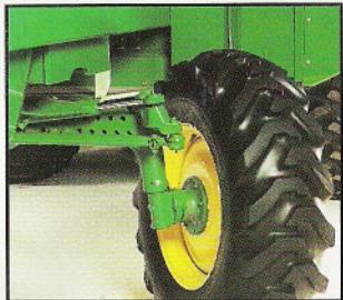
**Optional cleated guide tire improves steering control in muddy conditions.**
