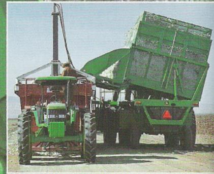
*Enjoy unprecedented unloading control with the new PRO-LIFT basket. Notice how the basket raises at an angle as the door lowers. With this unique design, the center of gravity remains very near the mid-point of the machine, providing exceptional stability... especially on uneven terrain.*
