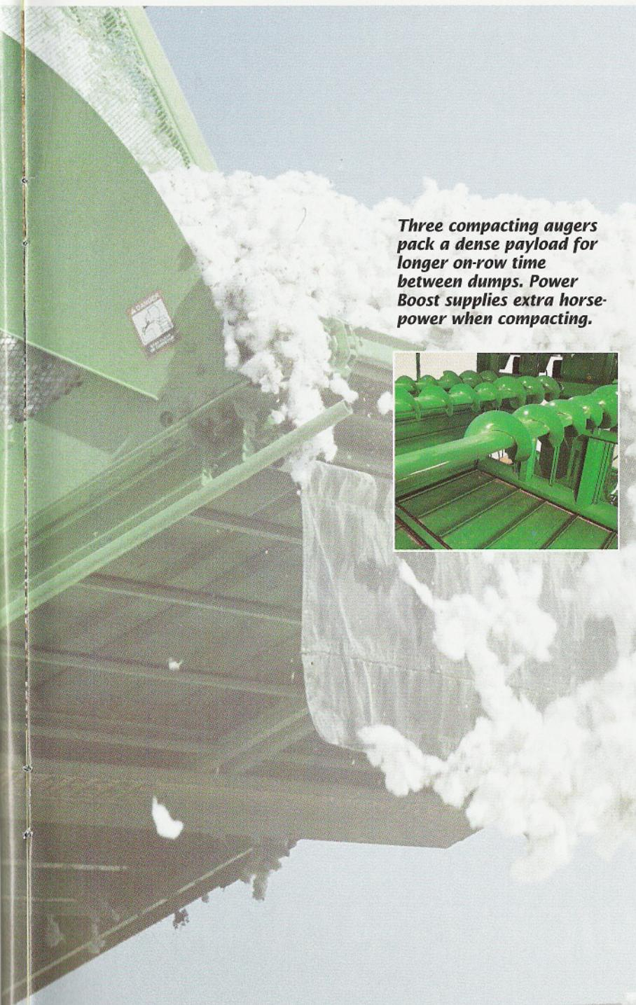
*Three compacting augers pack a dense payload for longer on-row time between dumps. Power Boost supplies extra horsepower when compacting.*
