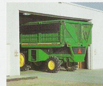
*Preparing to lower the PRO-LIFT basket is easy. First, fold in the duct side-shields, then hook up the duct support chains, pull the duct retaining pin (shown above), and*
