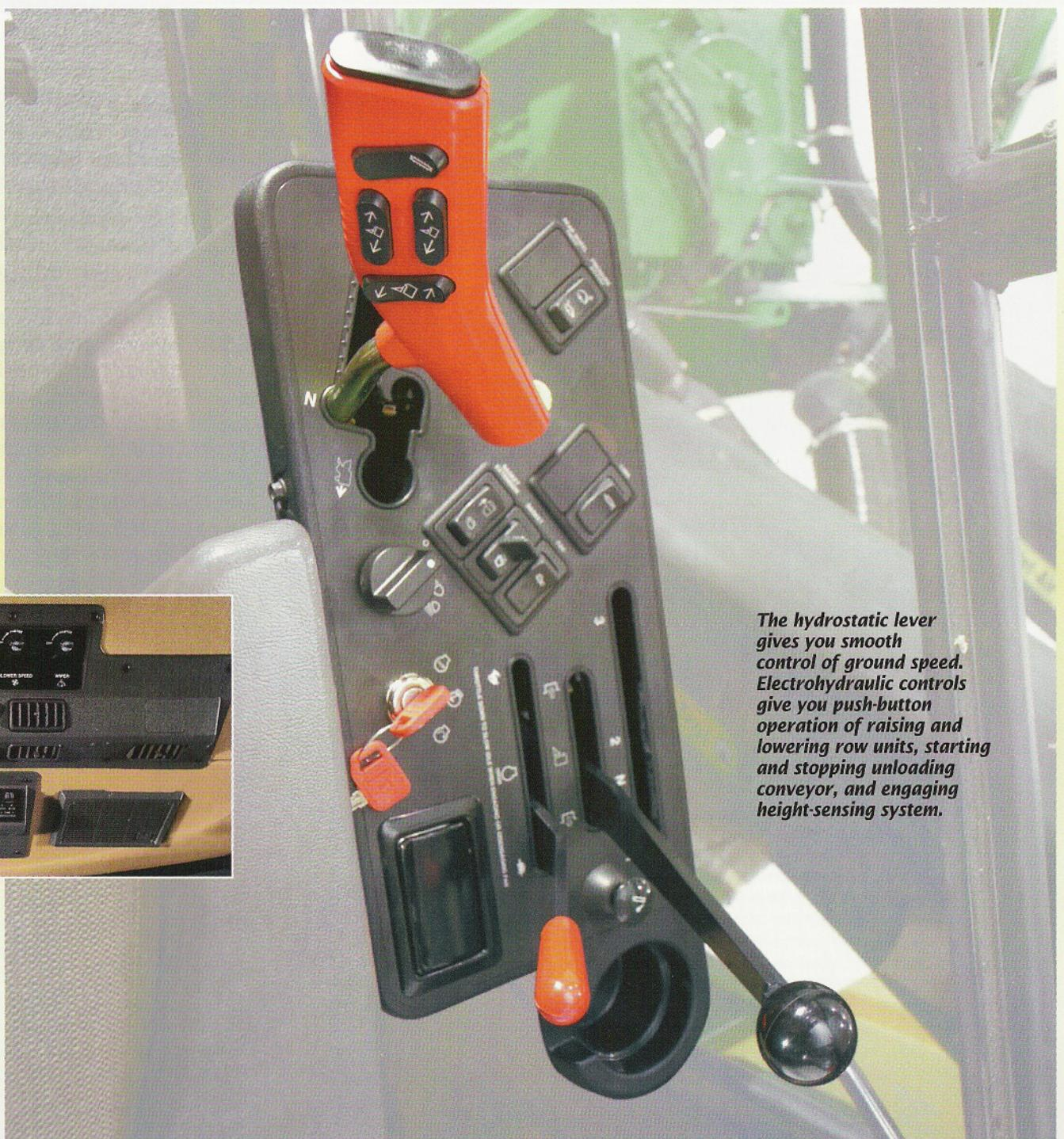
*The hydrostatic lever gives you smooth control of ground speed. Electrohydraulic controls give you push-button operation of raising and lowering row units, starting and stopping unloading conveyor, and engaging height-sensing system.*
