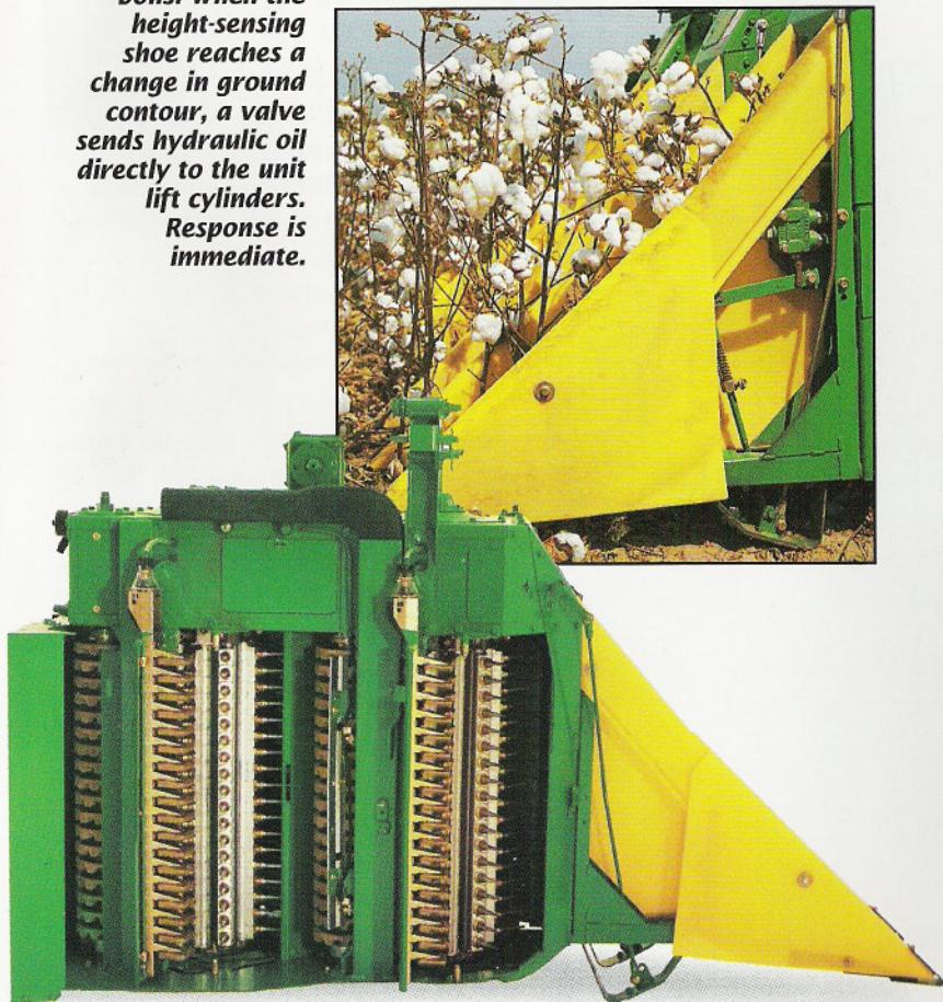
**New PRO-12 row units feature 12-bar front and rear drums, each with 18-spindle-high bars. Swing-out moistener columns make servicing a snap. (Please see pages 6 and 7 for more information about new PRO-SERIES row units.)**
