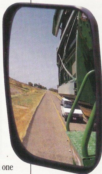
Rear mirrors on the 9965 Picker erase blind spots and give you a clear view to the sides and to the rear of the picker. They make transport safer and unloading easier.
