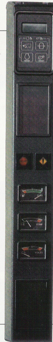
A simple digital readout provides engine and fan speed, moistener system pressure, and oil temperature. Problems with the picking units, such as plugging, are identified quickly with Harvest System monitors. A more-reliable sensing system alerts you at the first possible sign of plugging—long before it becomes a time-consuming cleanout.
