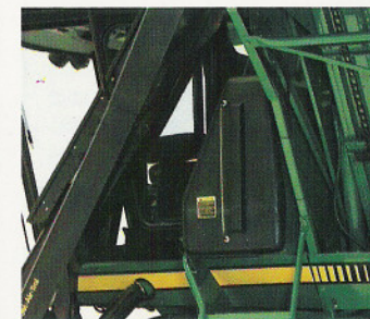
This 230-gallon solution tank on a 9950 allows operators to spend more time picking, less time refilling.
