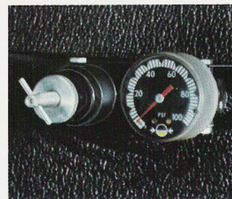
Flow regulator and an easy-to-see pressure gauge are at the left side of the seat.
