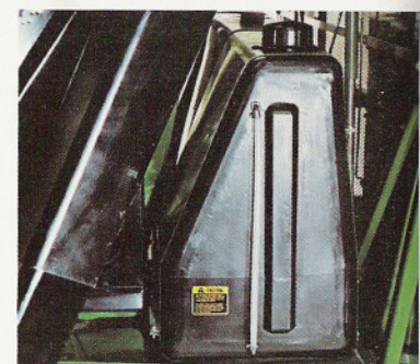
This 230-gallon solution tank on a 9940 allows operators to spend more time picking and less time refilling. It also increases on-row time.
