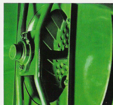
This 4100-rpm aerodynamic fan puts zip into the air delivery system, sailing cotton to the basket.
