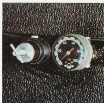
Flow regulator and pressure gauge are at the left side of the seat, to let operators monitor solution flow.
