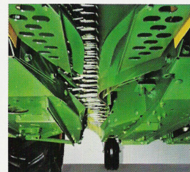
Row-unit bottom trash outlets behind the front picking drum allow trash and dirt to escape through the bottom. Outlets are also provided for the rear units.
