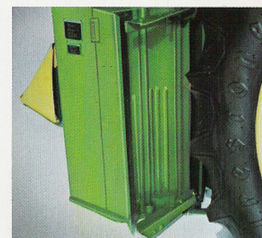
This front suction door is specifically designed for 12-bar drums front and rear. Louvers are located here where clean air can be sucked in and trash left outside. These doors increase air velocity around the front drum for a more efficient flow of air to send cotton to the basket faster.
