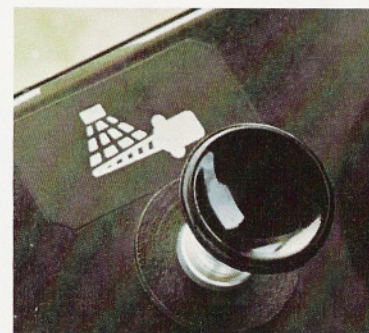
Pull this knob on the instrument panel and the pressurized flush system goes to work sending additional solution to the moistener pads.
