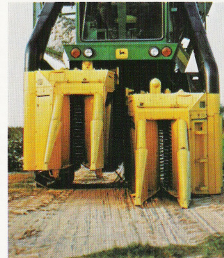
Push-type cylinders lift picking units—more reliable than pull-type cylinders because they're less likely to leak. The lift-arm linkage is designed to increase lift height, and exert less load on the rockshaft bearings.
