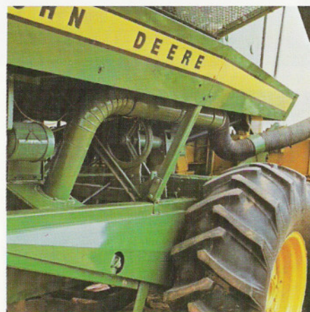
2. Sheet-metal tubing makes up a large portion of the air duct from the fan. This contributes to long life and fewer service and repair problems. The front portion is rubber tubing to provide the flexibility that is needed when picking units are raised and lowered.
