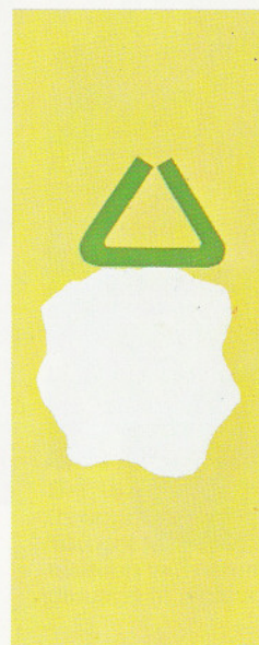
The cleaning-grate area on the 9900 basket (at right) has been increased by 29 percent over the 699 to provide maximum cleaning ability. The illustration shows the triangular shape of each of the cleaning-grate fingers. This shape protects your cotton quality by keeping seed from being cracked.
