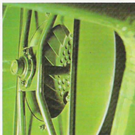
1. The aluminum rotor fan with aerodynamically designed fins produces a powerful air flow to handle the huge harvesting capacity of the 9900. This fan is designed to run quietly and smoothly.
