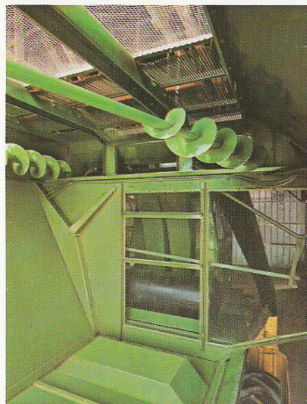
Two 6-foot-long, hydraulically driven augers (shown at left) gently distribute cotton to the back corners of the 608-cubic-foot basket to increase its holding capacity 20 percent.
