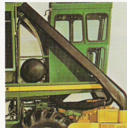
4. Straight conveyor ducts provide an obstruction-free ride for the cotton from the picking unit to the basket. There are no sharp edges or corners to damage cottonseed as it is carried through the ducts.
