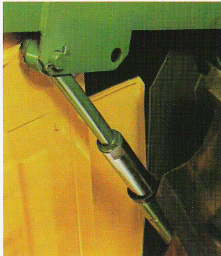
Push-type cylinders lift picking units—more reliable than pull-type cylinders because they're less likely to leak. The lift-arm linkage is designed to increase lift height, and exert less load on the rockshaft bearings.
