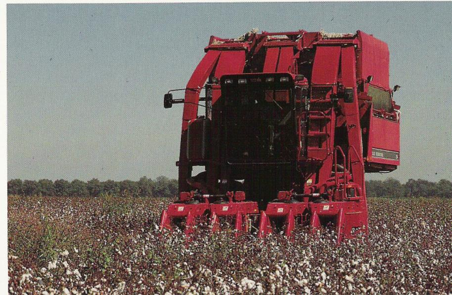
Monitor sensors, placed at strategic points from drums to the basket, keep an eye on the flow of cotton—unlike other systems that monitor air pressure. They also keep an eye on rotor and fan speeds. Should flow or the speed of a fan or rotor drop below normal, the system alerts the operator with both an audible alarm and a warning light.
