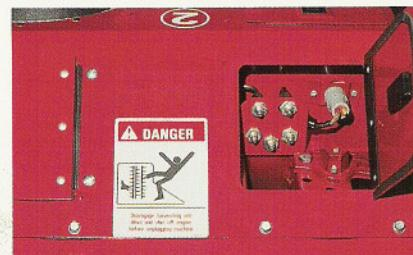
Standard equipment includes a chassis lube bank system with 19 fittings on the 2022 and 25 on the 2044.
