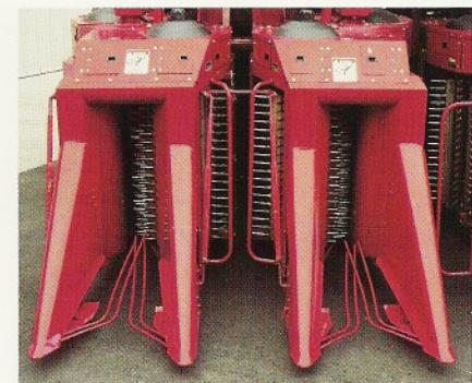
□ Automatic drum height sensing: Located up front on the plant lifters, they respond quickly to ground contour, reducing shoe bulldozing. Right- and left-hand row units operate independently, so one side can be raised while the other lowers. Helps you get more of those low-hanging bolls.
